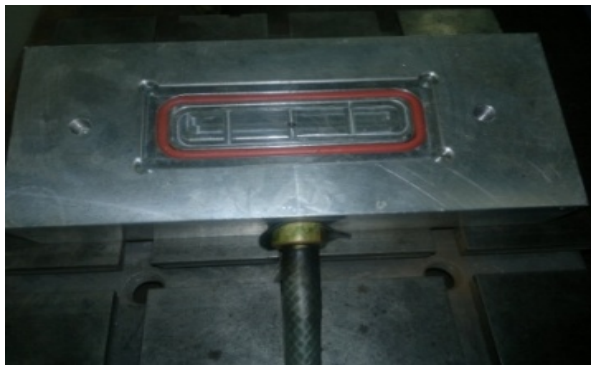
Fig. 2 Shop made vacuum fixture used for experiments [19]
