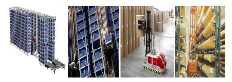
Fig. 11 Service robots – AGV with telescopic forks
