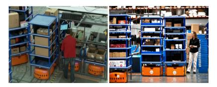
Fig. 14 Service robots - KIVA systems [23]
