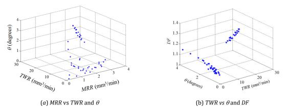
Fig. 4 Pareto-optimal solution obtained by MO-Jaya algorithm for EDM process in a single simulation run
