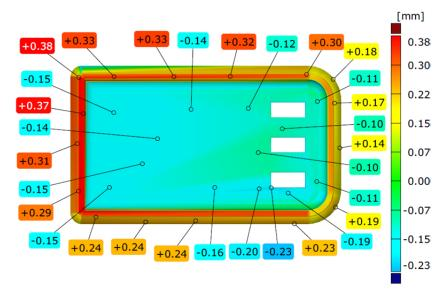
Fig. 12 Deviations of back camera cover - rear view
