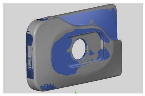
Fig. 6 Original STL (blue) and scanned front cover (grey) aligned in GOM Inspect
