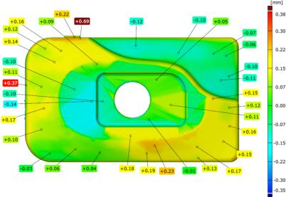
Fig. 8 Deviations of front camera cover - front view
