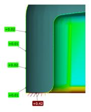
**Fig. 15** Detail of section with minimum deviation of scanned camera casing model
