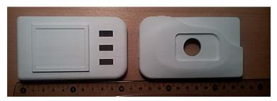
Fig. 2 3D printed models of camera casing
