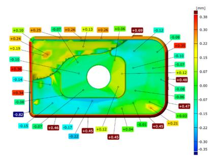
Fig. 10 Deviations of front camera cover - rear view
