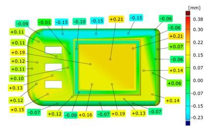
Fig. 11 Deviations of back camera cover - front view
