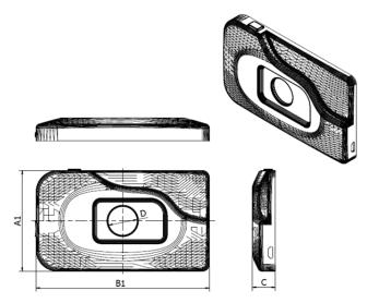
Fig. 3 Measured dimensions of original front cover
