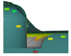
**Fig. 13** Detail of section with maximum deviation of scanned camera casing model
