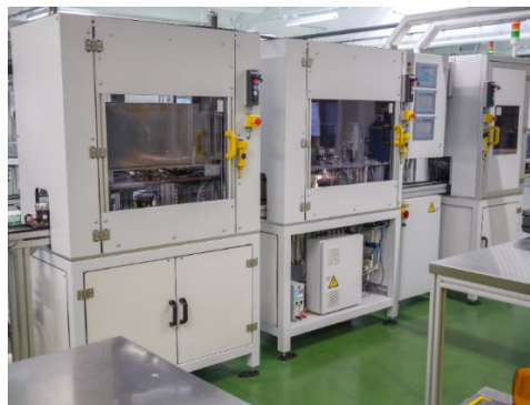
Fig. 2 Modular EoL quality inspection system
